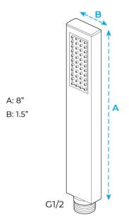
The minimum required water pressure is 0.05 MPa (0.5 bar). Flow rate 2.5 GPM (9.5 LPM).
